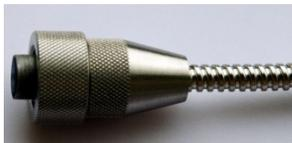
**TM0704-XX:** Stainless steel MIL connector with armored XX meters cable, 4.83mm diameter. Operating temperature range goes up to 150°C (300°F), Maximum Length is 10 meters.
