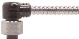
**TM0705-XX:** Cornered MIL connector with armored XX meters cable, 4.83mm diameter. Operating temperature range goes up to 120°C (250°F) , Maximum Length is 10 meters
